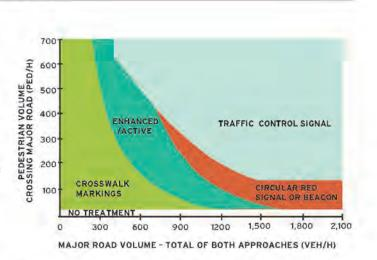
Figure 2-7. Example Guidelines for Pedestrian Crossing Treatments adapted from NCHRP 562 (Fig. A.5), Calculations assume 34 ft (10.4 m) Pavement, 35 mi/h (55 km/h), 3.5 ft/s (1.1 m/s), Walking Speed.
